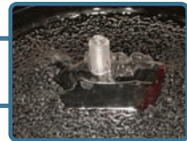
Fig.7b Baseplate & cylinder after thermoforming.
