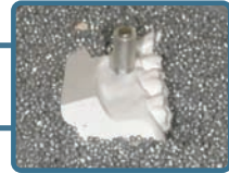
Fig.7a Model placed in pressure forming machine with guide cylinder in vertical position.
