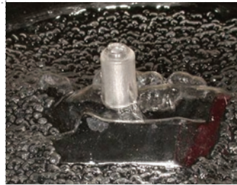
Fig.7b Baseplate & cylinder after thermoforming.
